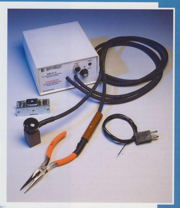
The high arc temperatures generated by the Weld-X<sup>™</sup> easily fuse all standard thermocouple materials, including platinum and tungsten. Wires can be welded in pairs in gages of #20 or finer, and individually for gages as heavy as #16.
